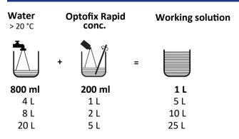
For fixing in machines working solution and replenisher are identical.
