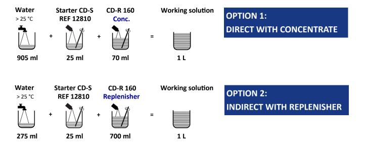
Corresponding to the size of the respective colour developer working tank, the quantities for water, Starter CD-S and CD-R 160 concentrate, resp. CD-R 160 replenisher are to be multiplied.
